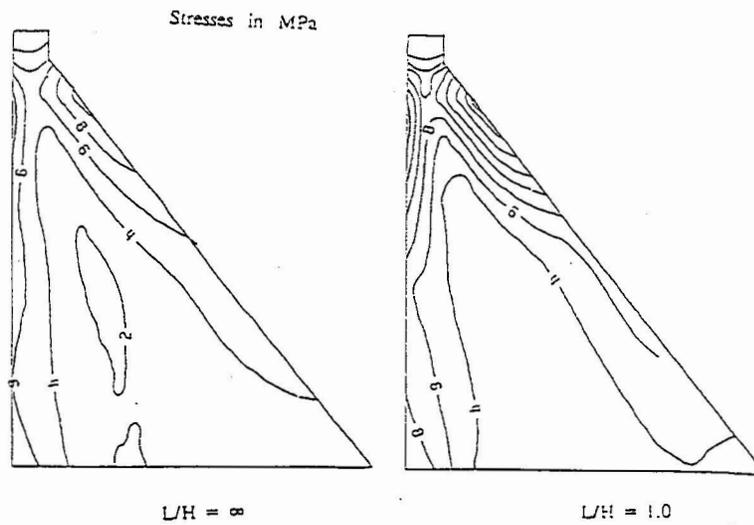
Figure 3 - Dynamic Tensile Stress Profile, Saguenay Earthquake Record
