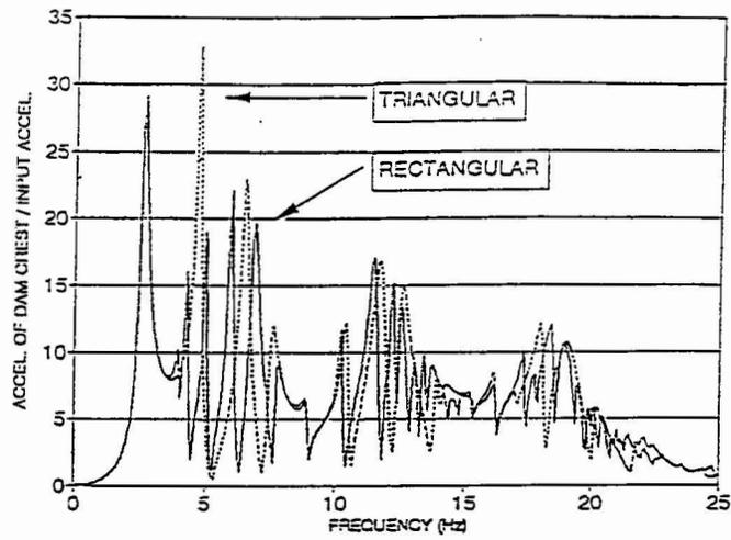
Figure 4 - Fourier Representation of monolith's response for a rectangular and triangular reservoir geometry
