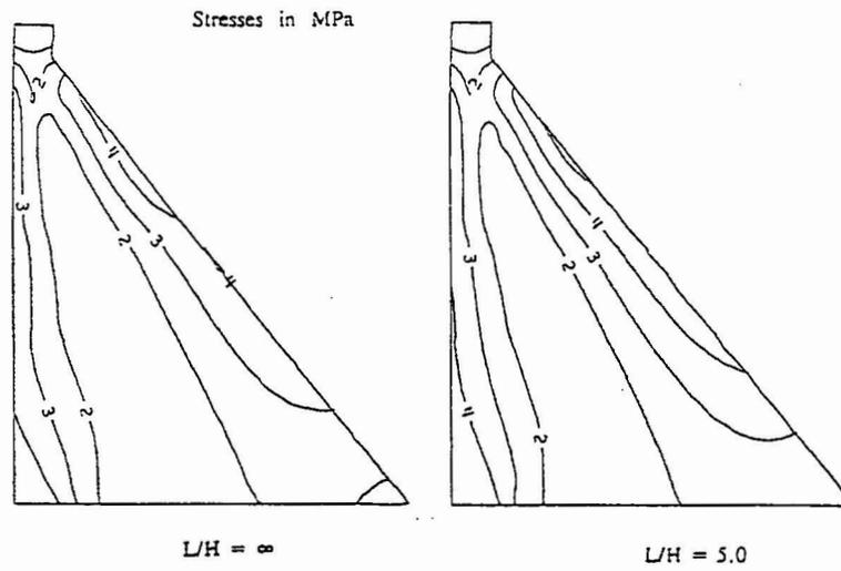
Figure 2 - Dynamic Tensile Stress Profile, Imperial Valley Earthquake Record
